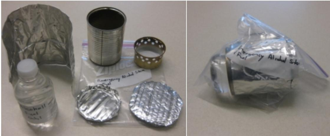
For more information about alcohol stoves in general, try searching the web for “alcohol stoves”. For the particular design that I used, search for “cat food can alcohol stove”. I started with an empty cat food can, cleaned it, then used a paper punch to put two lines of holes around the top. In under five minutes, I had a working alcohol stove.
